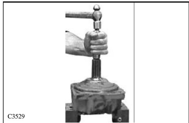
17 At this point the shaft should drop straight downwards. The shaft seal can now be removed and replaced. It can not be removed in any other way. (fig. C3530)
