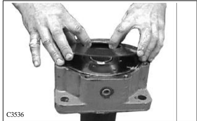
6 Install brake cover and cross tighten all screws to final torque specification of 65ft/lbs. (fig. C3537)
