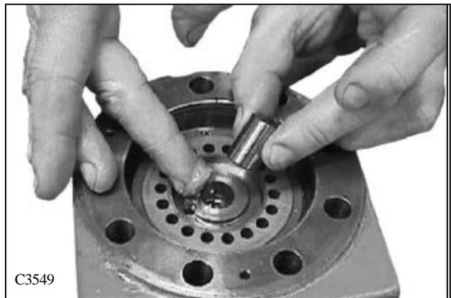
19 Since the motor has been disassembled, the guide pins will locate ports in the offset position. To align with the drain and brake ports, turn the section until correct port alignment is made (fig. C3550).
