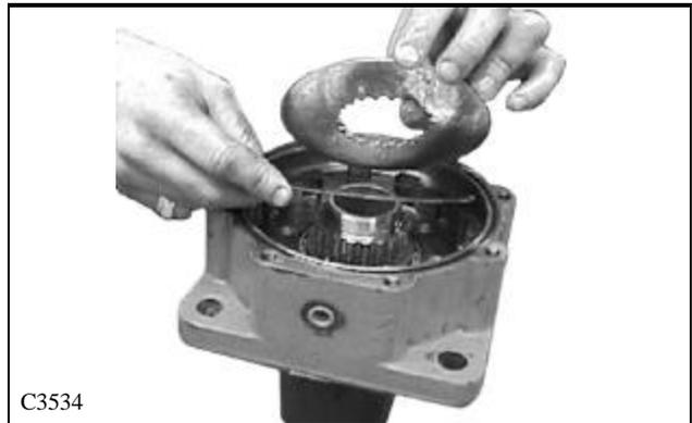
4 Install the piston after all of the disks have been inserted. There will be air trapped, but this will escape when the spring and cover are installed. (fig. C3535)
