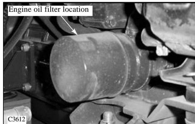
5 Lubricate the new oil filter O-ring seal with engine oil and install to the engine hand tightened.
