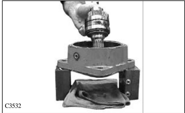
2 Install bearing retaining ring and tighten with Torx drive to 7ft/lbs. (fig. C3533)
