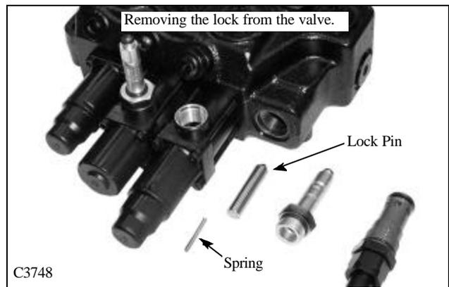
3. Remove the spring return detent kit and spring center cap locks. (fig. C3749)
