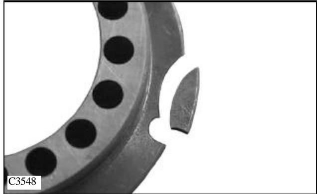
18 With the balance plate in the proper position and tapped down to seat, apply some vaseline or grease to prevent the spacer from falling out when installed onto the motor (fig. C3549).
